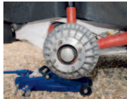
...while the rear Superfin drums are supported by coloured AVO adjustable dampers.
