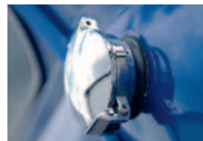
The Aston chrome flip filler cap matches the chrome hinges, wipers, grille and bumpers.
