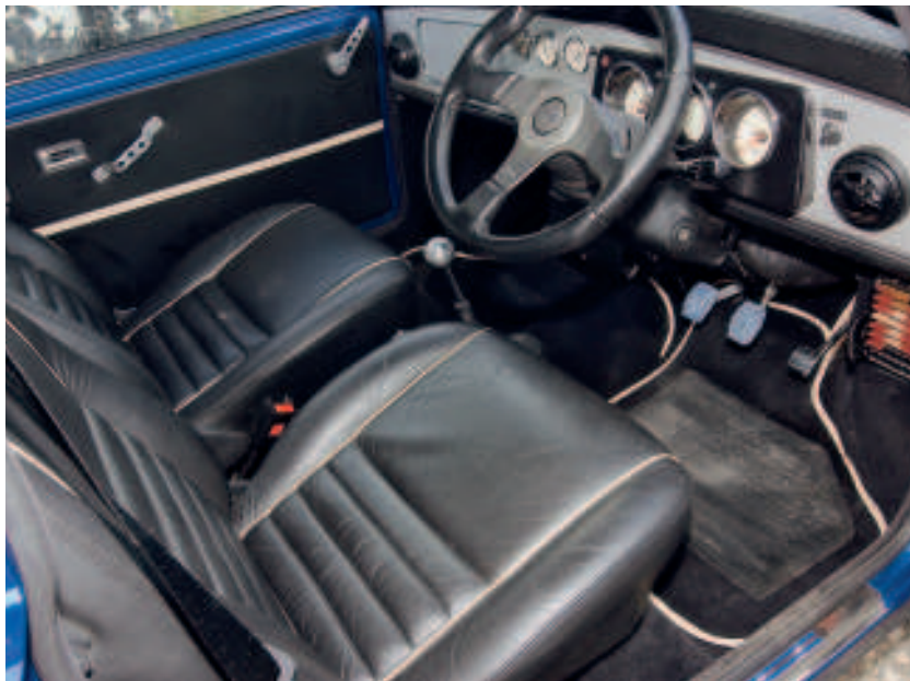
Full leather Cooper seats were fitted for a more luxurious ride, along with a set of Wilton carpets.
