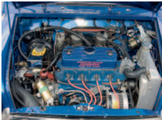
The overbored 1399cc engine has been fitted with a Stage 3 kit and three-core radiator to cool the engine.
